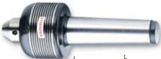
1. Shaft uses material SKD11:through vacuum heat tretment, it is even more durale, hardness is as high as (HRC60°±2°)and satisfied wear-resistance. Main body is made of SCM21 material.
