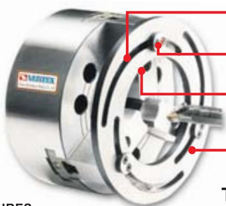
The size can be adjusted against the helical slot.
