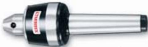
1. Center shaft is made of SKS3 material under vacuum heating treatment to provide higher rigidity (HRC60°+2°) and satisfied wear-resistance.
