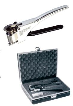
**The Model B Tester** is designed to cover the hardness of aluminum alloys from the 1100 to the 7075 series. The 20 graduations on the Webster dial indicator covers the range between 25 and 110 on the Rockwell E Scale.
