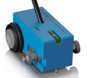
The purpose of scratch hardness tests is to determine the resistance of coating materials or lacquers to scratch effects on the surface. This test is of particular value for furniture or vehicle lacquers, but is also a useful aid in the development of synthetic resins or other film forming materials.
